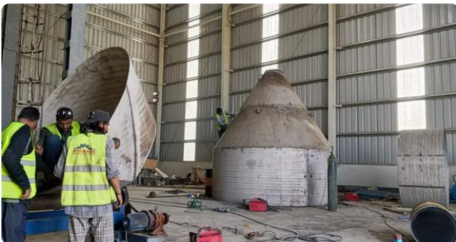
SS cone and shell fabrication
